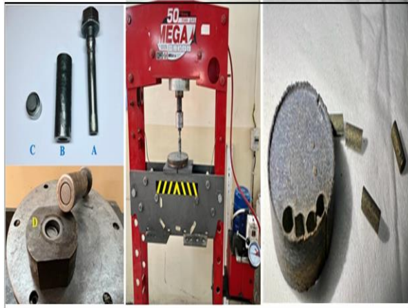
Figure 1: (Left) Mold used in the study (A: The punch, B: The die, C: The base, D: the ejector base) (Middle) hydraulic press (MEGA, Spain) (Right) sample preparation using wire-cut machine.
